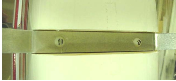
Figure 2 Main gear mounted
