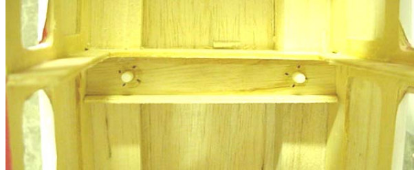
Figure 3 Inside view of mounting points with 1/4-20 nylon hardware installed
