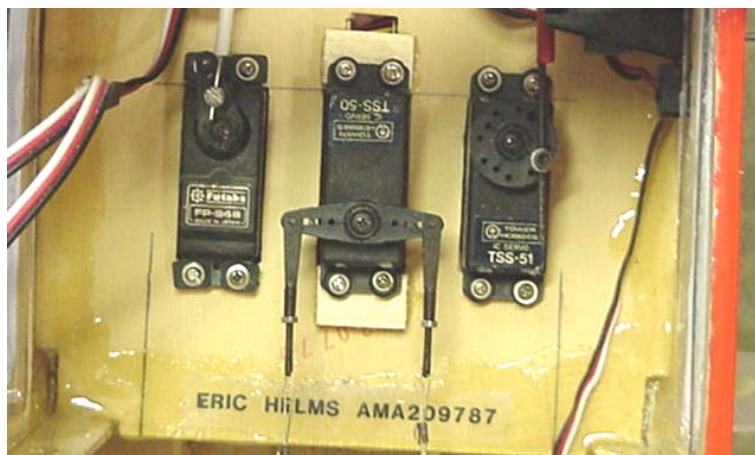
Figure 5 Pull-pull cables installed on servo cross-arm
