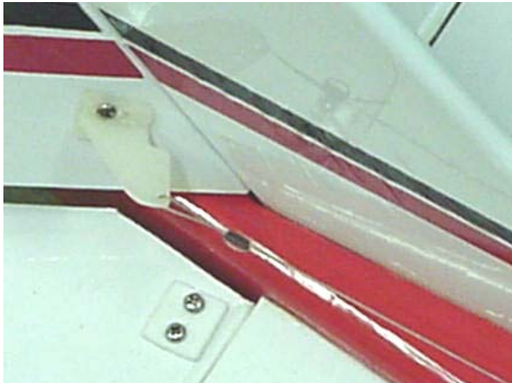
Figure 6 Pull-pull cables installed on servo rudder
